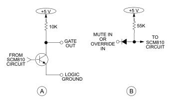
LOGIC EQUIVALENT CIRCUIT DIAGRAMS FIGURE 10
